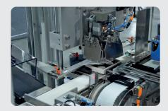
**Modular Sealer** Optional modular sealer unit allows for quick and compact sealing operations.
