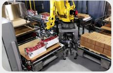
Provides automatic delivery of empty pallets to loading station, providing uninterrupted operation when combined with multiple stations.
