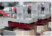
**Press on tab** Positively guided can turning enables reproducible follow-up operations.
