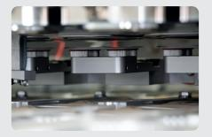
Lid transfer The lid is transferred directly into the sealing tool with perfect positioning on the can.
