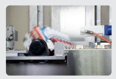
**Can turner** After a turn in the can turner, the flap presser bends the flap under the edge.
