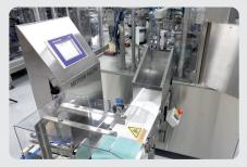
**QC & Check Weighing** Ability to add quality control features such as weighing technologies or cameras.
