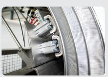
**Piece by piece** In the destacker system, cans are separated and transferred to the transport rail.
