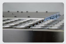
**Clean walking beam** The transport system prevents product contamination from being carried over.
